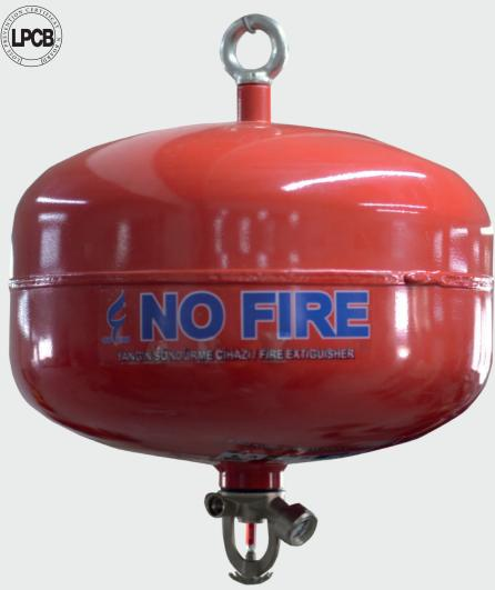
These automatic powder fire extinguishers are designed for installation in larger areas where an increased discharge range is required. When the temperature reaches 68°C the extinguisher unit automatically discharges, releasing the powder agent and smothering the fire. The units are ideal for applications such as engine compartments, engine rooms and storage areas.
